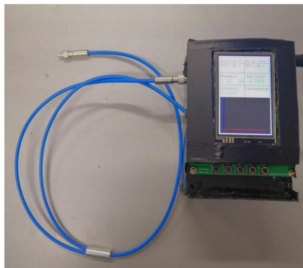
Figure 3. Physical view of the corneal fluorescence measurement device.
